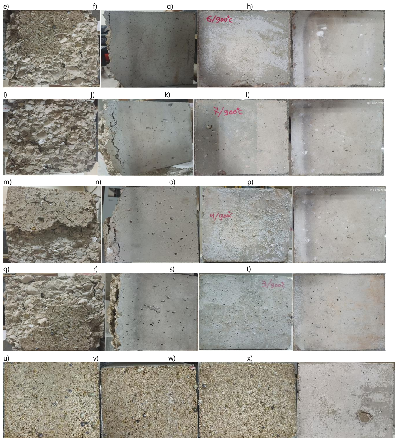
Figure 8: Performance of concrete blocks against maximum high temperature. Mix I to Mix V (c, d, g, h, k, l, o, p, s, and t) and x – explosive spalling of aggregates for Mix III at max. 900 °C. u, v, w – melting of aggregates for Mix II, Mix III, and Mix IV at 1050 °C. Mix I to Mix V (a, b, e, f, i, j, m, n, q, and r) at max. 1200 °C.
